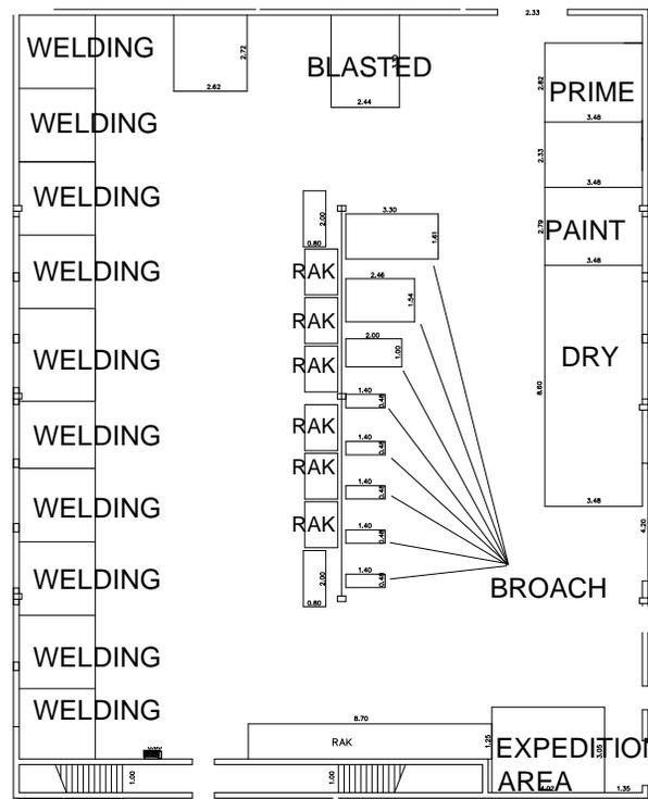
Picture 1 – Functional layout example in a metalworking industry
