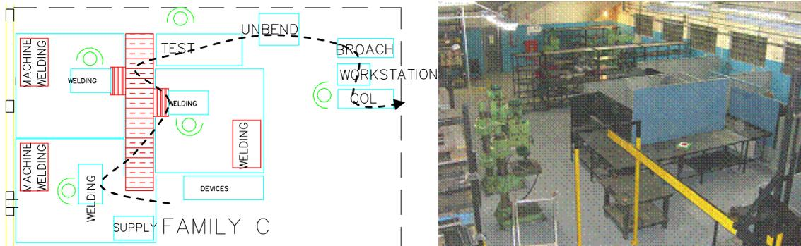
Picture 2 – Cellular layout example in a metalworking industry
