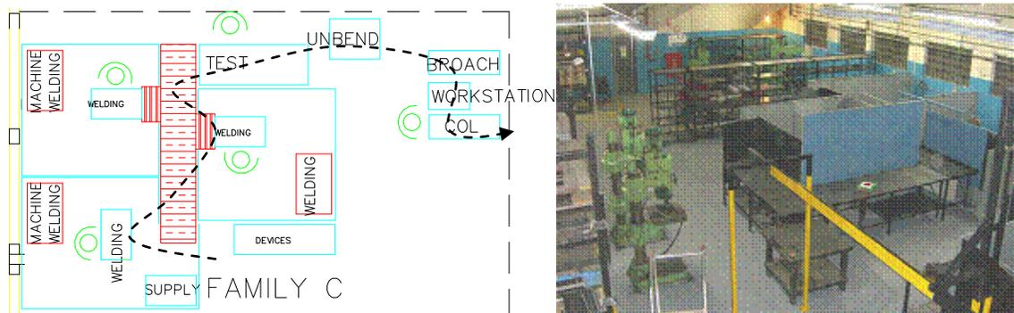
Picture 2 – Cellular layout example in a metalworking industry
